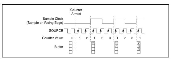
Figure 7-5 shows an example of non-cumulative buffered edge counting.
